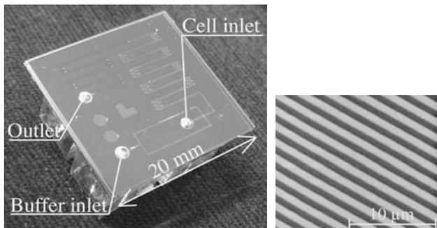
Figure 3: (a) Photo of the present device, (b) SEM image of the oblique grooves.
