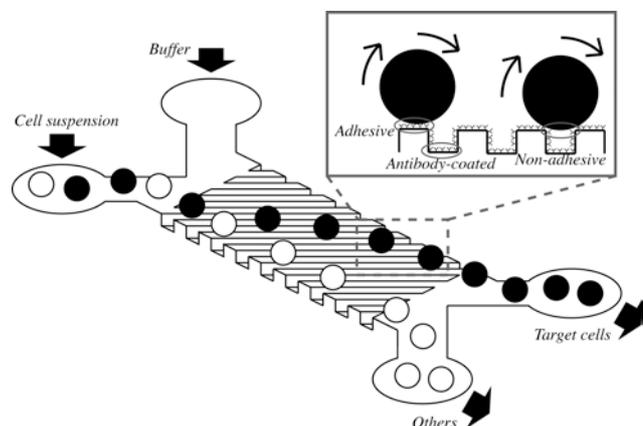
Figure 1: Cell separation principle using oblique antibody patterns.
