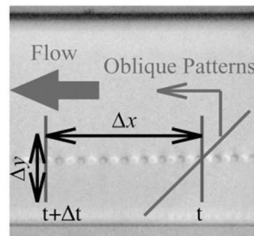
Figure 5: Microscopic measurement of micro beads velocity and displacement.
