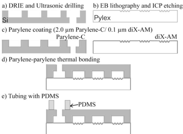
Figure 2: Microfabrication process.
