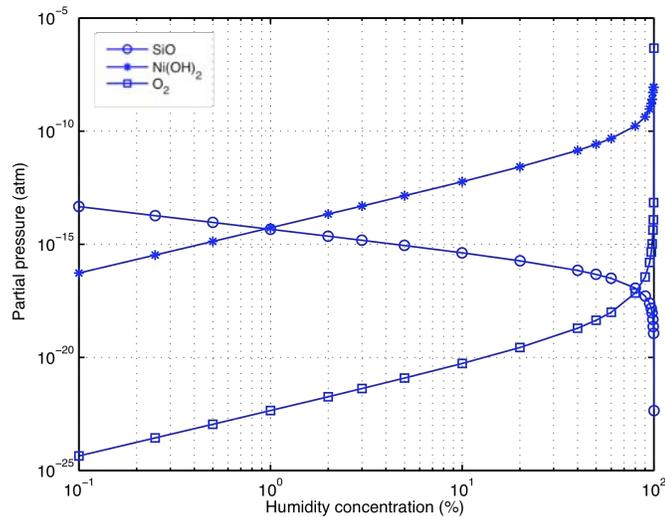
Figure 5. Partial pressure of gaseous phases versus humidity in hydrogen.
