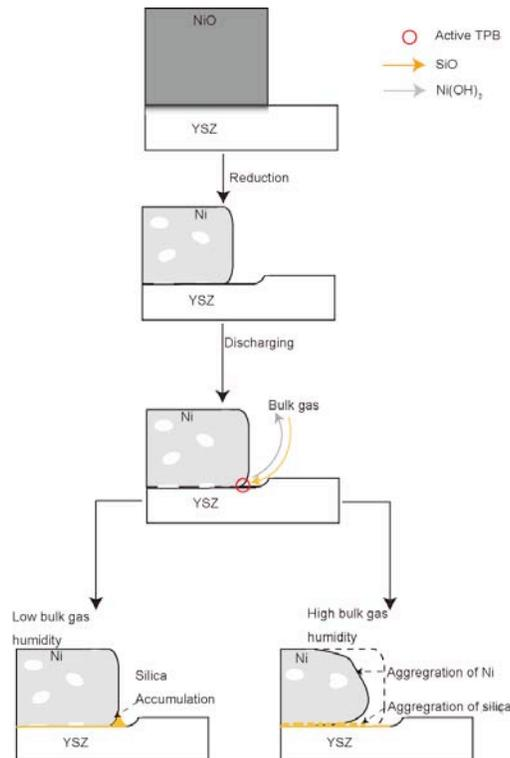
Figure 6. Ni-YSZ interface change mechanism illustration.
