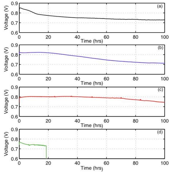
Figure 1. Anode-to-reference terminal voltage within (a) dry, (b) 3% H<sub>2</sub>O, (c) 10% H<sub>2</sub>O and (d) 30% H<sub>2</sub>O hydrogen with a discharge current density of 200 mA/cm<sup>2</sup>.
