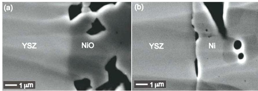
Figure 3. (a) YSZ-NiO interface after sintering. (b) YSZ-Ni interface after reduction.
