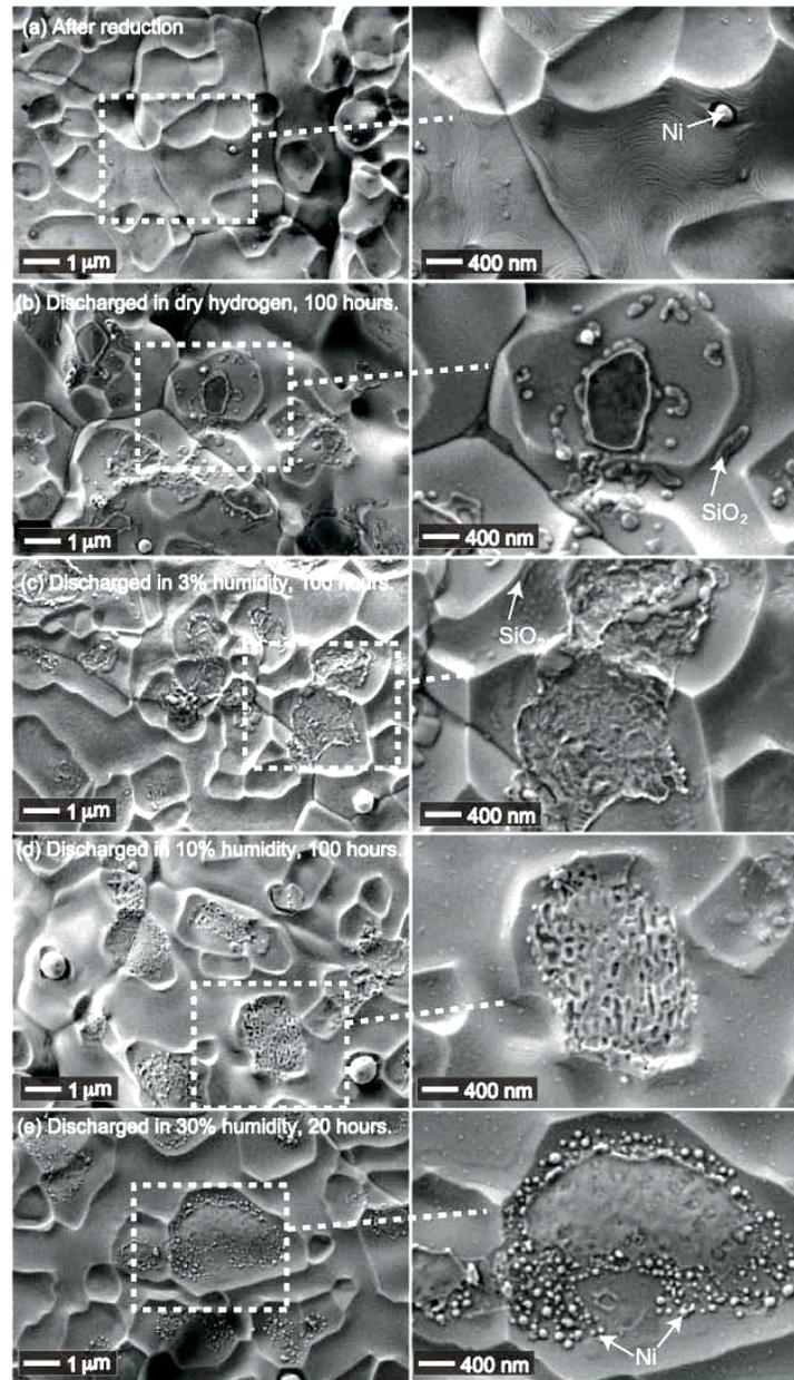
Figure 4. Top views of YSZ-Ni interfaces (a) After reduction, (b)-(e) after discharge corresponding to Figure 1. (With Ni anode mechanically stripped off from YSZ surface.)
