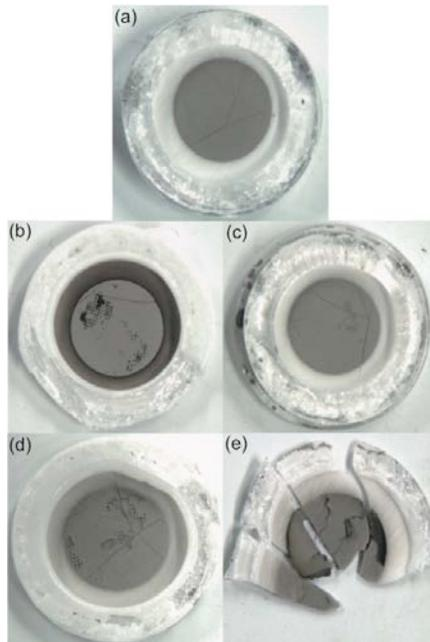
Figure 2. Top views of the anodes. (a) Just after reduction, (b)-(e) after discharge corresponding to Figure 1 (a)-(d).
