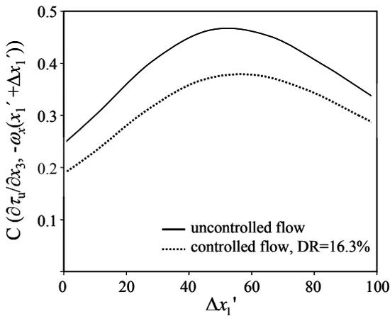
Figure 4: Spatial correlation,  $C$ , between the spanwise gradient of the streamwise wall shear stress and the streamwise vorticity at different downstream locations for an uncontrolled flow and a controlled flow according to equation (9). The normalization is based on the inner variables of each flow.
