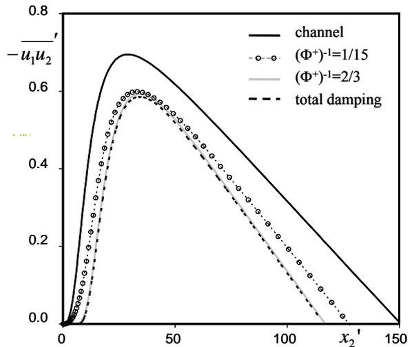
Figure 2: Reynolds stresses of controlled flows ( $y_d^+=10$ ) in comparison with the Reynolds stresses of the uncontrolled channel flow and of the total damping case (Iwamoto et al., 2005). The dash indicates that the normalization is based on the inner variables of each controlled flow.
