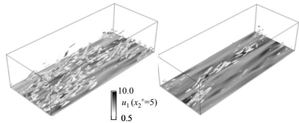
Figure 9: Flow visualization of the uncontrolled channel flow at  $Re_\tau=150$  (left) and the controlled case ( $S=17.6\%$ ) according to equation 9 (right). The visualization of the streamwise vortices is based on isosurfaces for which the second invariant of the deformation tensor is given by  $\Pi^+=0.02$ .
