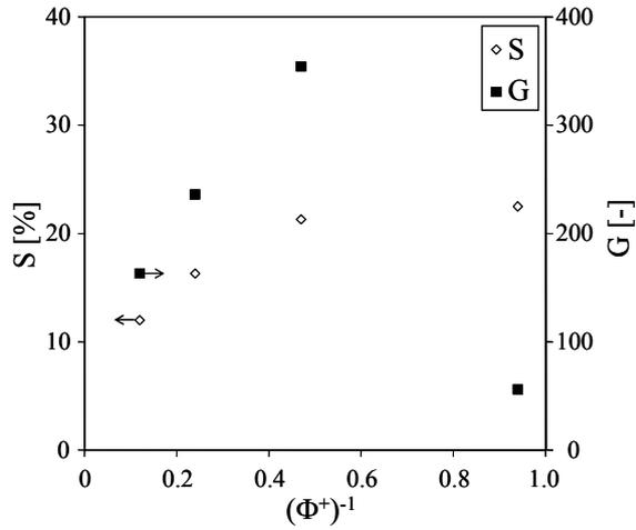
Figure 6: Effect of the forcing strength  $(\Phi^+)^{-1}$  on  $S$  and  $G$  for flow the flow control loop given by equation (9).
