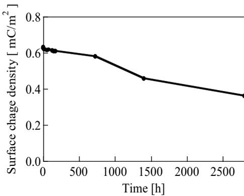
Figure 3. Time trace of mean surface charge density.
