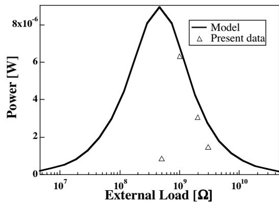
Figure 7. Power output versus external load.
