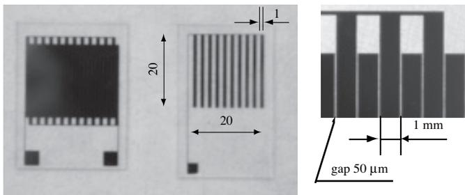
Figure 4. Patterned counter electrode(left), electret (middle), and close-up view of the counter electrode (right).
