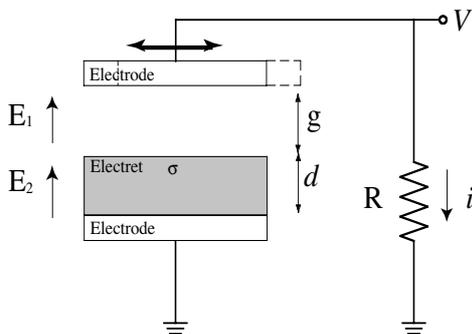
Figure 1. Model of electret generator.
