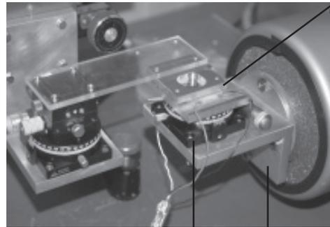
Electrode chip on rotation stage Shaker
