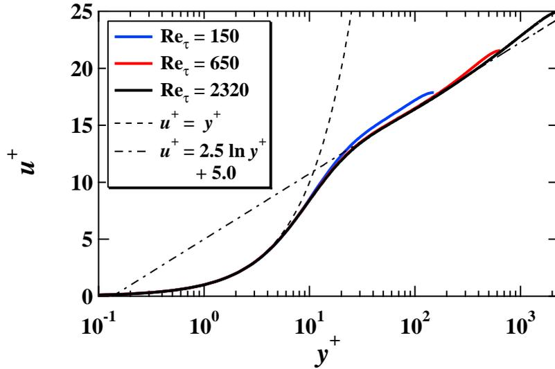
Fig. 1 Mean streamwise velocity profiles at  $Re_\tau = 2320$ , 650 [12], and 150 [12].
