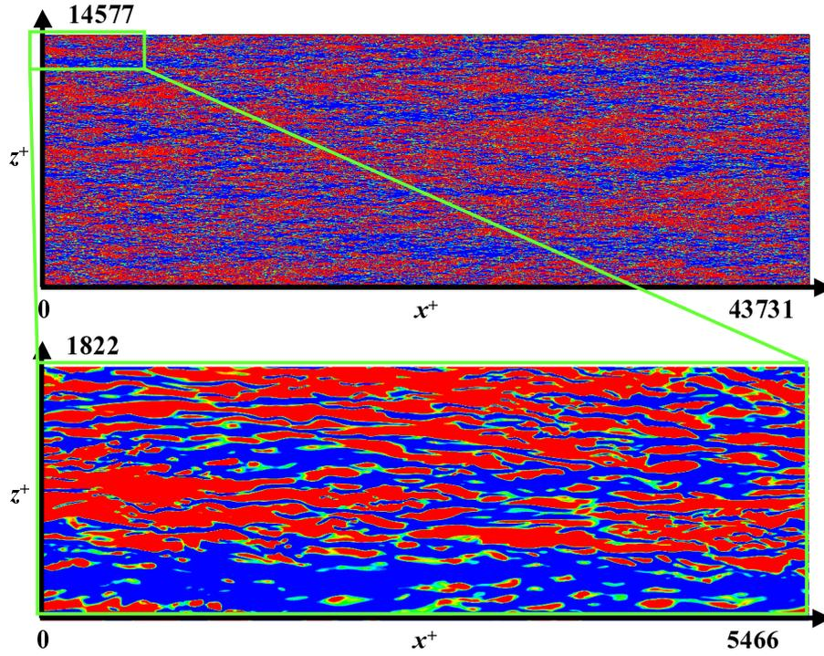
Fig. 3 Plane views of instantaneous near-wall velocity field at  $y^+ \approx 11$ . Contours of the streamwise velocity fluctuation, blue to red,  $u'^+ = -1$  to  $u'^+ = 1$ . Total computational volume is 43731 and 14577 wall units in the  $x$ - and  $z$ -directions, respectively.
