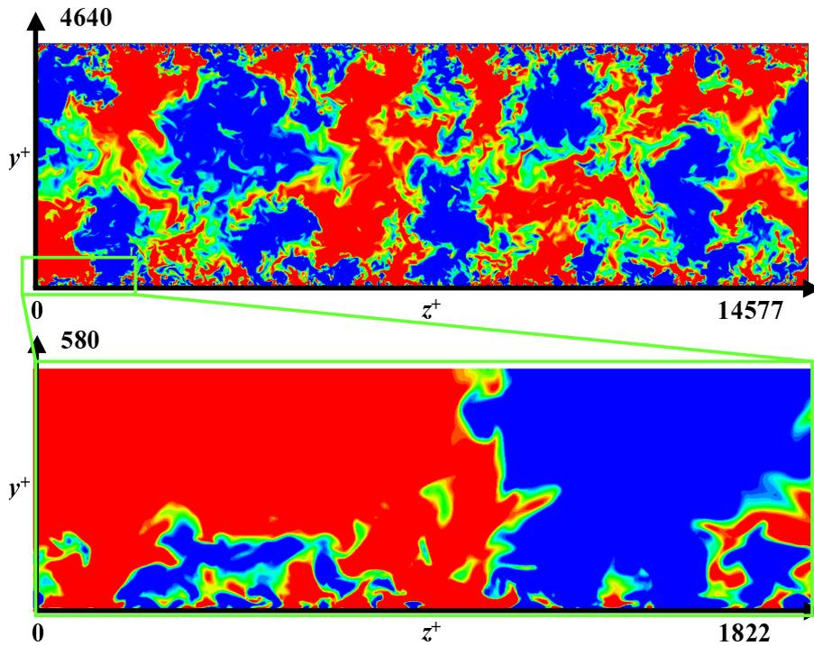
Fig. 4 Cross views of instantaneous velocity field. Contours of the streamwise velocity fluctuation, blue to red,  $u'^+ = -1$  to  $u'^+ = 1$ . Total computational volume is 4640 and 14577 wall units in the  $y$ - and  $z$ -directions, respectively.
