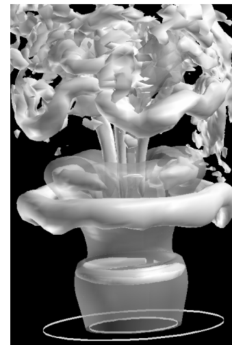
Fig. 16 Instantaneous vortical structures (white opaque) and scalar iso-surface (gray transparent).
