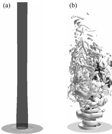
Fig. 14 Instantaneous vortical structures (white) and scalar concentration distributions (black). (a) natural jet, (b) controlled jet ( St_{ctrl} = 1 , \varepsilon = 0.0125 ).
