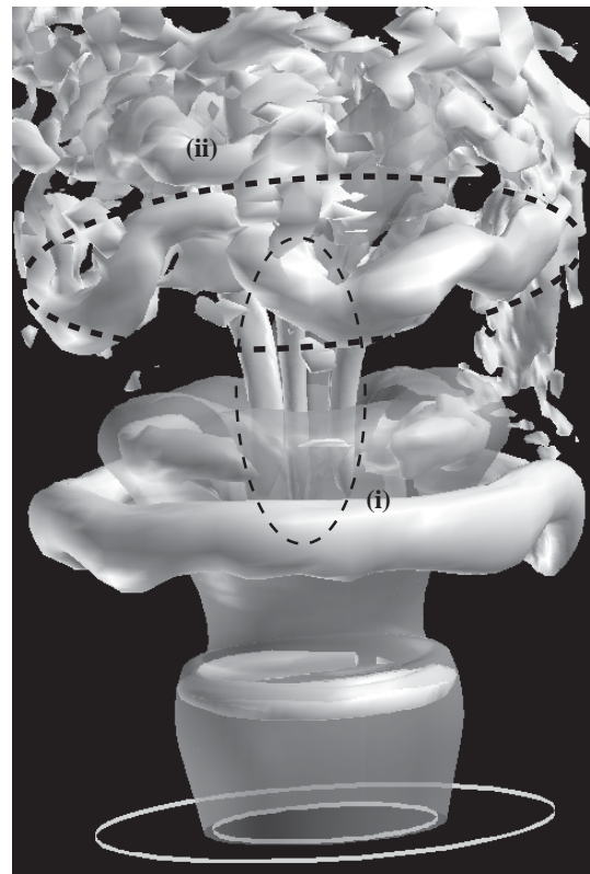
Figure 13: Instantaneous vortical structures (white opaque) and scalar isosurface (gray transparent).
