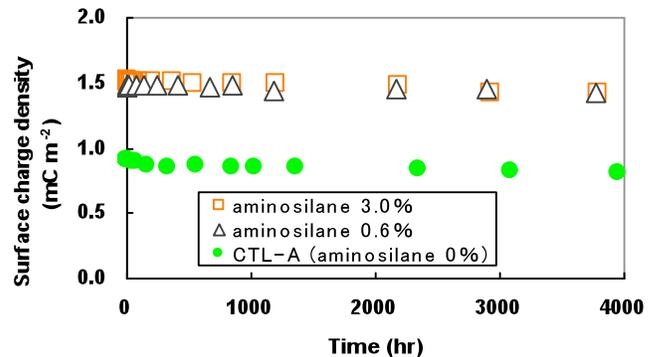
Fig. 2. Time trace of the surface charge density of aminosilane-doped CYTOP (aminosilane 0.6 wt%, and 3.0 wt% ; film thickness:15μm)
