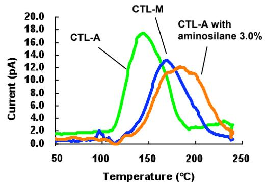
Fig. 3. TSD spectra of CTL-A, CTL-M, and aminosilane-doped CYTOP (aminosilane 3.0 wt% ; film thickness:15μm)
