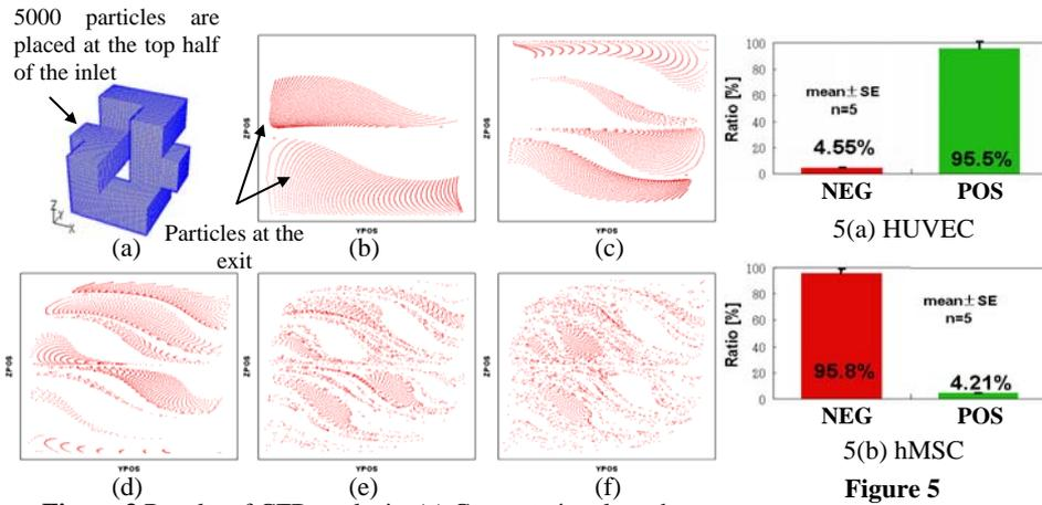
**Figure 3** Results of CFD analysis, (a) Computational mesh, Particle distribution at the exit of (b) 1<sup>st</sup>, (c) 2<sup>nd</sup>, (d) 3<sup>rd</sup>, (e) 6<sup>th</sup>, and (f) 9<sup>th</sup> unit.
