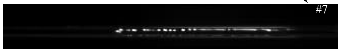
Fig. 3 Explosive boiling from the superheated liquid near the seventh thermocouple (same experimental run as in Fig. 2).
