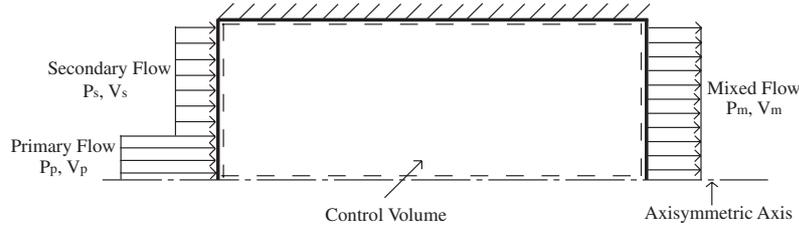
**Figure 3.** Control volume in quasi-1D calculation.
