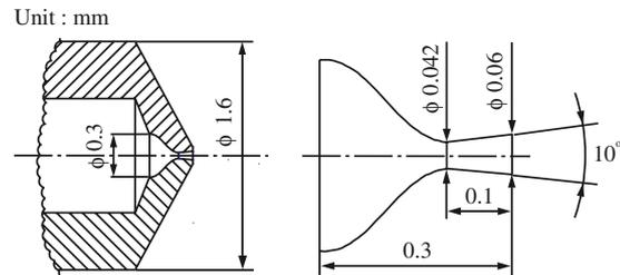
Figure 8. Schematic of the micro nozzle.
