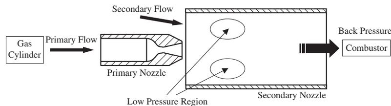
**Figure 2.** Schematic of ejector for micro combustor.
