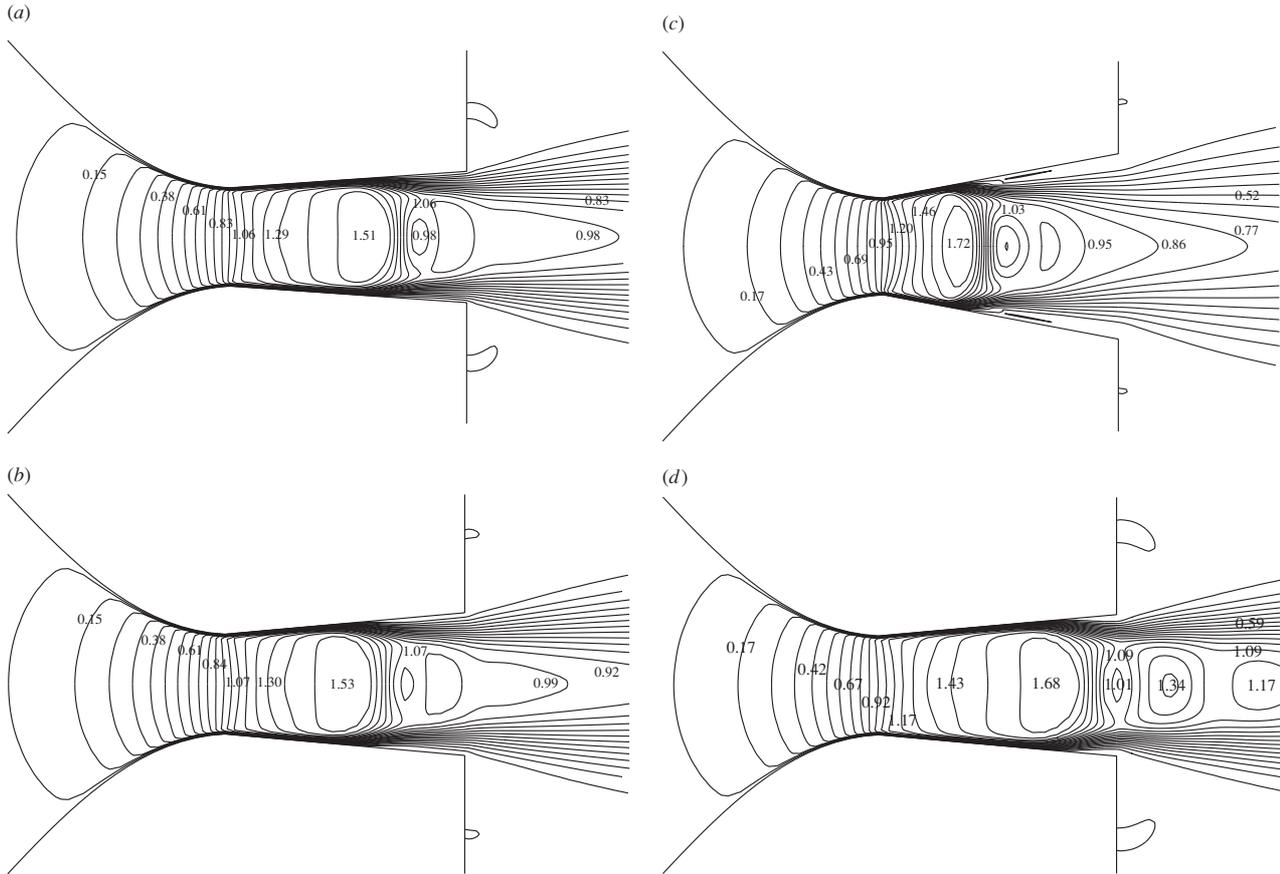
**Figure 4.** Contours of the Mach number in the primary nozzles with different configurations. (a) Nozzle design with an expansion angle of  $8^\circ$ ,  $P_{TP} = 0.1$  MPa; (b) present design (expansion angle =  $10^\circ$ ),  $P_{TP} = 0.1$  MPa; (c) nozzle design with a expansion angle of  $21.5^\circ$ ,  $P_{TP} = 0.1$  MPa; (d) present design (expansion angle =  $10^\circ$ ),  $P_{TP} = 0.16$  MPa.
