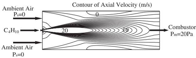
Figure 5. Contours of the axial velocity.
