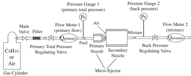
**Figure 10.** Experimental setup for the micro ejector.
