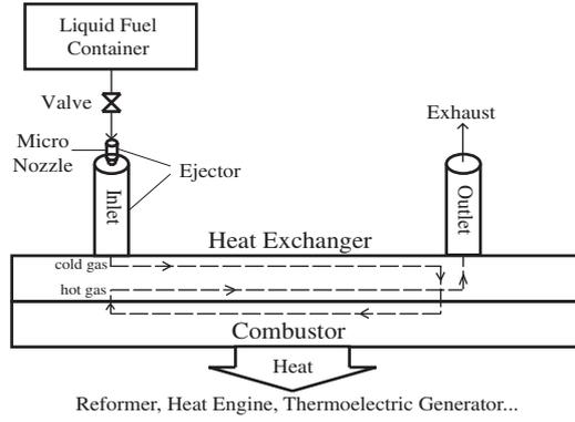
**Figure 1.** Micro heat generation system with ejector.
