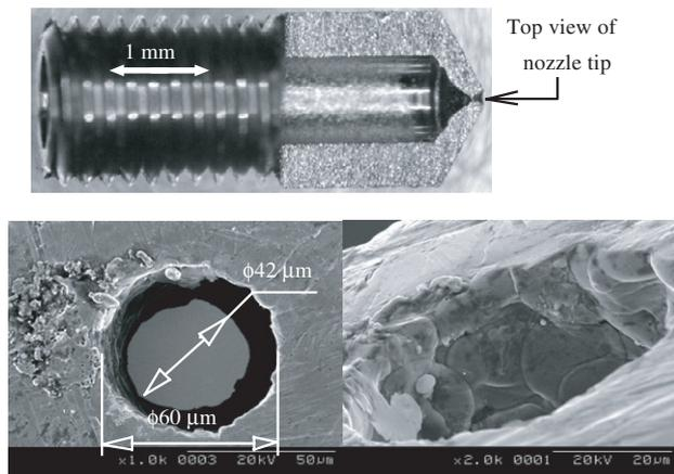
Figure 9. Microscopic image of micro nozzle (top), and SEM images of the nozzle tip: a top view (left) and a magnified view (right).
