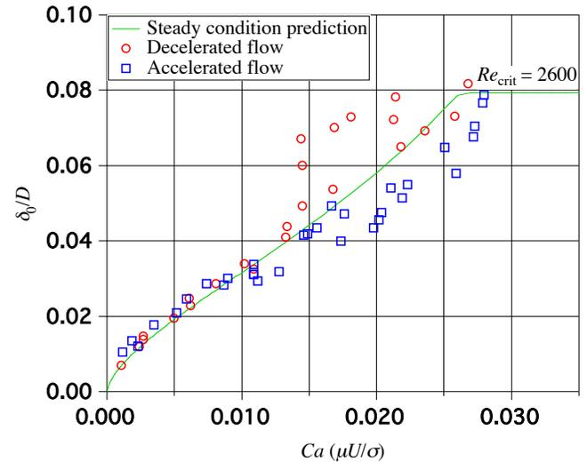
Fig. 10 Dimensionless liquid film thickness versus capillary number in oscillating flow.
