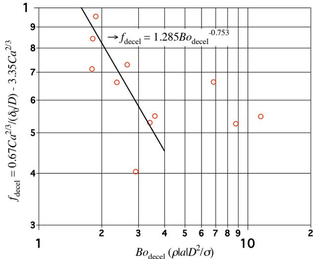
Fig. 8 Relation between  $f_{\text{decel}}$  and  $Bo_{\text{decel}}$ .
