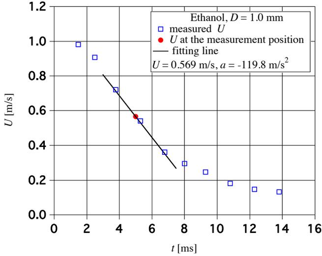
Fig. 4 Measured interface velocities in decelerated flow.
