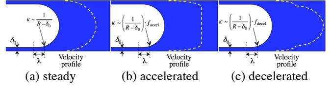
**Fig. 8** Schematics of velocity profile inside liquid slug under steady, accelerated and decelerated conditions.
