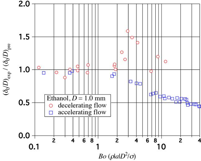
**Fig. 7** Ratio of measured liquid film thickness to predicted values in decelerating and accelerating flows.
