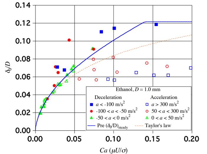
Fig. 6 Initial liquid film thickness in decelerating flow.
