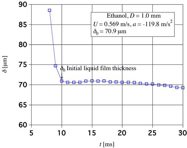
Fig. 5 Time variation of liquid film thickness.
