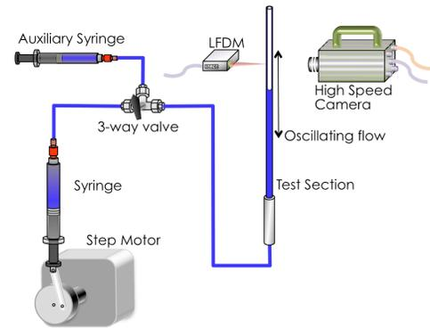
Fig. 9 Schematic diagram of the experimental setup for oscillating flow.
