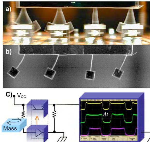
Figure 6: Parylene pendulum structures in resonance at  $60\ \text{Hz}$ . a) Long-exposure photo, b) Snap shot, c) Read-out circuit with the photointerrupters and output signals taken with a digital oscilloscope.
