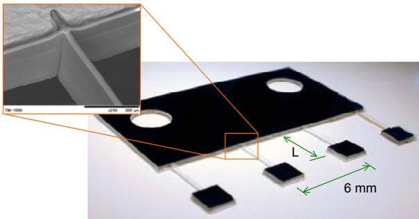
Figure 3: Test chip with 4 pendulums. Parylene beam width is  $30\ \mu\text{m}$ . Beam lengths ( $L$ ) from left to right are 4.0, 3.95, 3.9 and  $3.85\ \text{mm}$ . Dimension of the mass is  $2.0\ \text{mm} \times 2.0\ \text{mm}$ . The inset is a SEM image of the beam junction.
