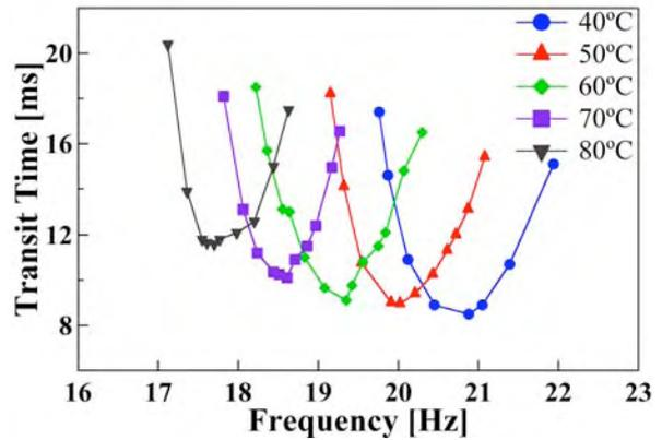
Figure 9: Frequency response of parylene-C pendulums for different temperatures. The minimum transit time of each curve corresponds to the resonant frequency.
