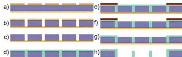
Figure 2: Process flow of parylene high-aspect-ratio springs.
