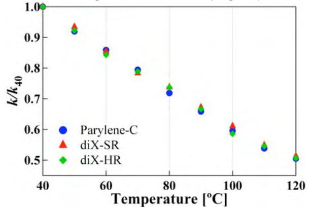
Figure 10: Spring constant normalized with the value at 40 °C. Three different parylene materials have the same TCY of 0.6 %/K.
