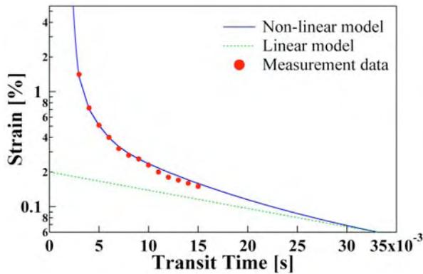
Figure 7: Comparison of the maximum strain at the point of maximum stress on deflecting beams. Beam length is 4 mm and oscillation frequency is 30 Hz.
