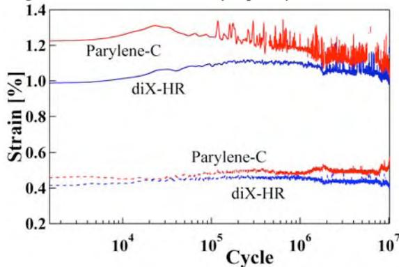
Figure 8: Experimental results for the cyclic load tests of parylene-C/diX-HR beams.
