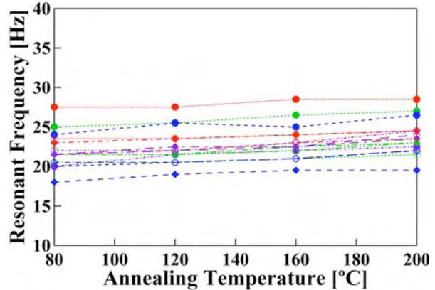
Figure 11: Effect of short-term thermal annealing on the resonant frequency: solid lines, diX-HR pendulums; dashed lines, parylene-C pendulums. Data for 4 pendulums with different beam lengths are plotted for both parylene-C and diX-HR.
