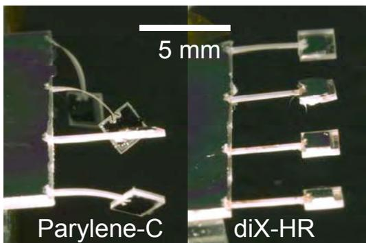
Figure 4: Free-standing parylene-C (left) and diX-HR (right) beams after thermal annealing at  $140\ \text{°C}$  for 5 hours. Beam width and height are respectively  $30\ \mu\text{m}$  and  $350\ \mu\text{m}$ .
