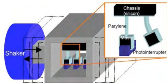
Figure 1: Measurement set-up with on-line strain monitoring.
