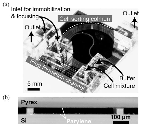
Fig. 4 (a) Microfabricated adhesion-based cell sorting device, (b) SEM image of the parylene micro channel cross section.
