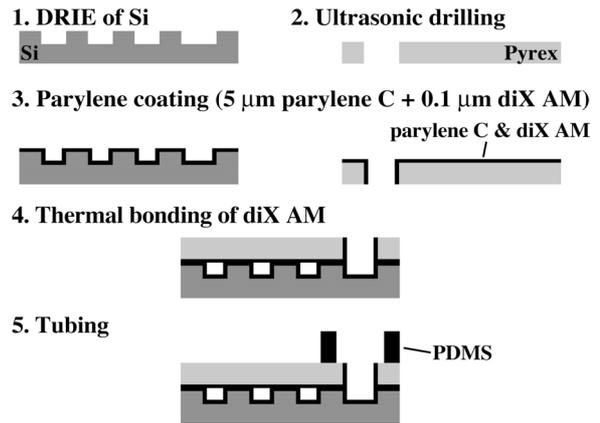
Fig. 3 Microfabrication process of diX AM channel structure.
