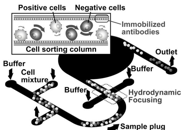
Fig. 1 Schematic of the adhesion-based cell sorter.
